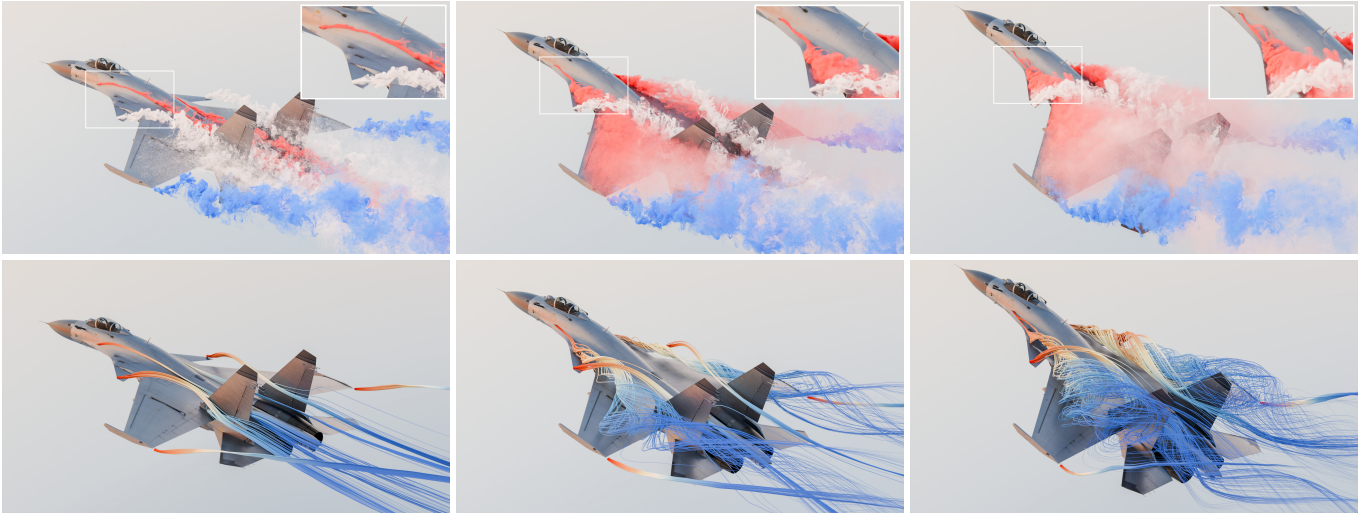
Fig. 16. Visual simulation of a maneuvering fighter jet. To demonstrate the scheme's reliability in handling complex geometries, we conducted simulations of a fighter aircraft across a range of angles of attack ( \text{AoA} = 8^\circ, 16^\circ, 22^\circ ). Flow field visualization was achieved via particle tracers released from the leading edges, as well as the trailing edges of both the canards and main wings. The top row presents the particle rendering results, whereas the bottom row depicts the corresponding time-averaged streamline distributions. These results clearly demonstrate that our scheme captures the intricate multiscale vortex dynamics and the complex mutual interactions between the canard and main wing vortices. Notably, the high-fidelity resolution of small-scale flow structures induces intense turbulent mixing, as clearly evidenced by the highly mixed particle distributions trailing the main wing.
